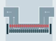
Transit-time principle for inline flow measurement
