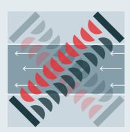
Transit-time principle for clamp-on flow measurement
