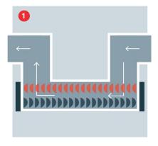
SONOFLOW flow meters use the transit-time ultrasound method to accurately determine the flow rate. The sensor measures the time of flight of the ultrasonic wave with and against the streaming liquid.
