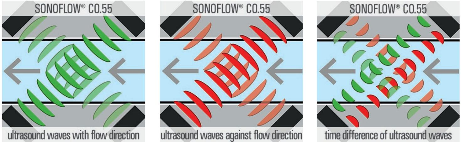
The transit times in and against the flow direction of a medium are measured with high precision by time-to-digital converters. In the direction of flow, the transit time of an ultrasonic wave is faster than in the opposite way. Like a sport boat, which moves in and against the flow direction of a river. A simple difference of both times allows a determination of the flow. In the case of the SONOFLOW® CO.55 sensor, the transmitted sound waves are sloped through
