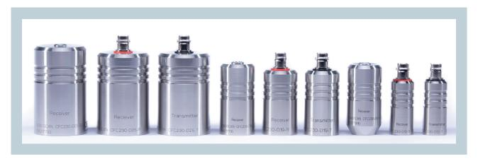
The ultrasonic SONOSCAN CFC230 transducers with a frequency of 230 kHz are used for air-coupled testing with the inspection system SONOAIR. The probes are available with apertures of 12.5 mm | 19 mm | 25 mm. Transmitter and receiver are adjusted separately. The receivers are available with integrated preamplifier (several discrete gain steps up to 80 dB) or as passive version.
