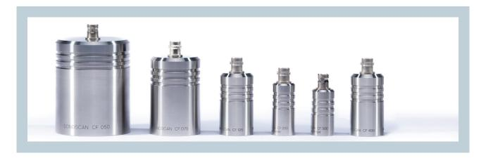
The probes of the SONOSCAN CF series have been designed for couplant-free material testing with the inspection system SONOAIR. The probes in stainless steel housing are available in frequencies from 50 to 400 kHz.
